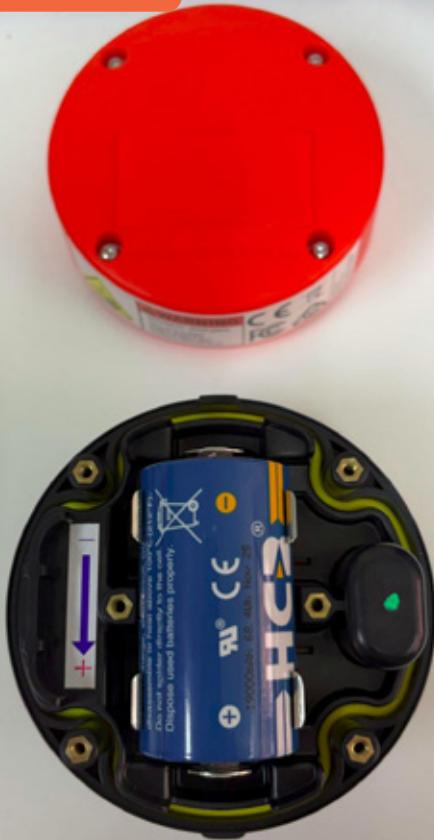
Unscrew the 4 M3 x 20mm captive T10 Torx screws from the orange lid external enclosure screw holes using a T10 Hex bit (this bit can be found at hardware stores or online).
