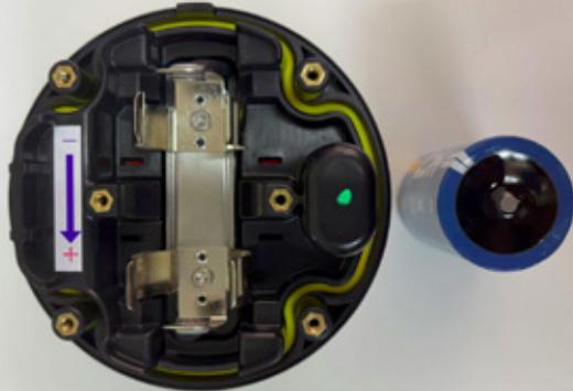
At this stage, remove the battery from the battery bucket.
