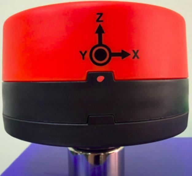
Place the orange lid back onto the housing, ensuring the lid and housing positioning notch line up.
