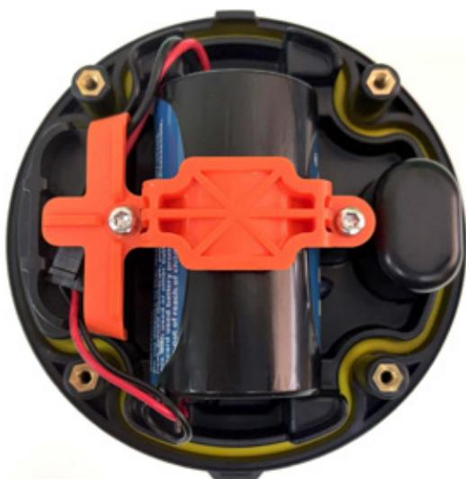
Unscrew the 4 M3 x 20mm captive T10 Torx screws from the orange lid external enclosure screw holes using a T10 Hex bit (this bit can be found at hardware stores or online).
