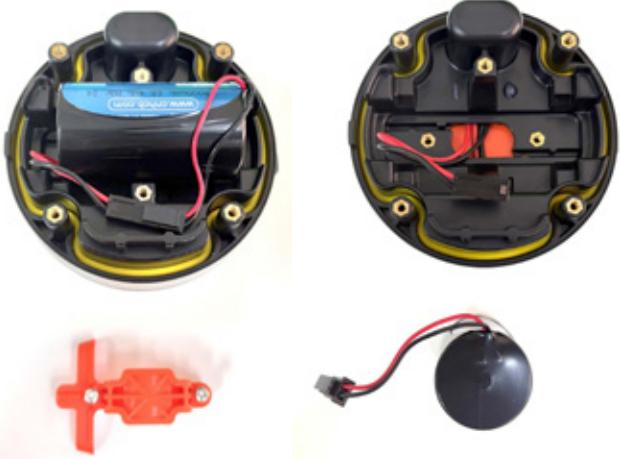
At this stage, unscrew the two M3 Torx T10 screws from the orange bracket and remove it to gain access to the battery.
