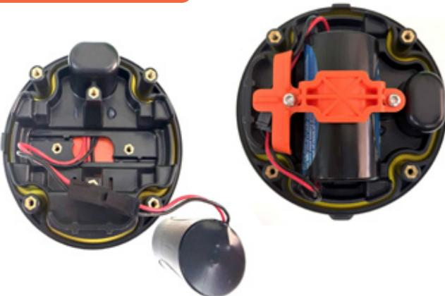
Orientate the new battery connector head so that the battery connector can be plugged in correctly (red wire aligning with the other red wire, black wire aligning with the other black wire), and then place the battery within the housing.
