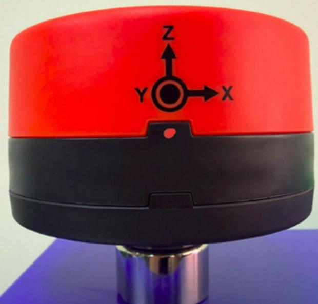
Place the orange lid back onto the housing, ensuring the lid and housing positioning notch line up.
